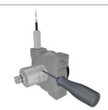
By tightening (approx. 2 Nm) the outer radial screw with a 2.5 mm hex wrench the encoder housing will be clamped to the sensor housing and secured from twisting. The system is now ready to be used.
