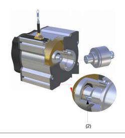
By tightening (1.5 Nm) the radial screw the encoder will be clamped and secured from twisting. Please use a hexagon screwdriver, size 3.
